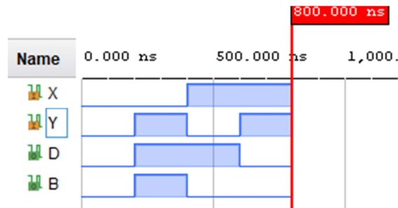
Figure 3.6: Functional verification of half subtractor truth table
